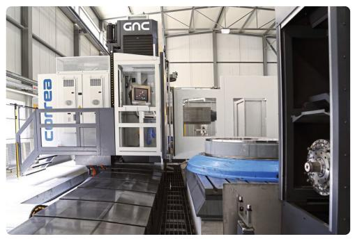
Hydro's milling machine AXIA is equiped with automatic head changer for two heads.
